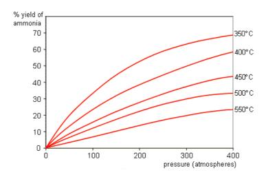
The Haber process is carried out at a **temperature of 450°C**, pressure of **200 atm** and in the presence an iron catalyst.
