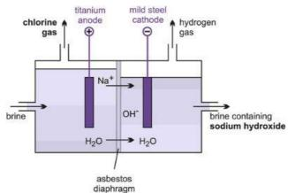
Brine is made with **concentrated sodium chloride solution**. The diaphragm allows for particles like Na<sup>+</sup> and H<sub>2</sub>O molecules to pass through but does not allow negatively charged ions like OH<sup>-</sup> and Cl<sup>-</sup> to pass through.
