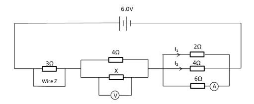
a) The ammeter registered a reading of 0.5A. Determine the  $I_1$  &  $I_2$ . [2]
