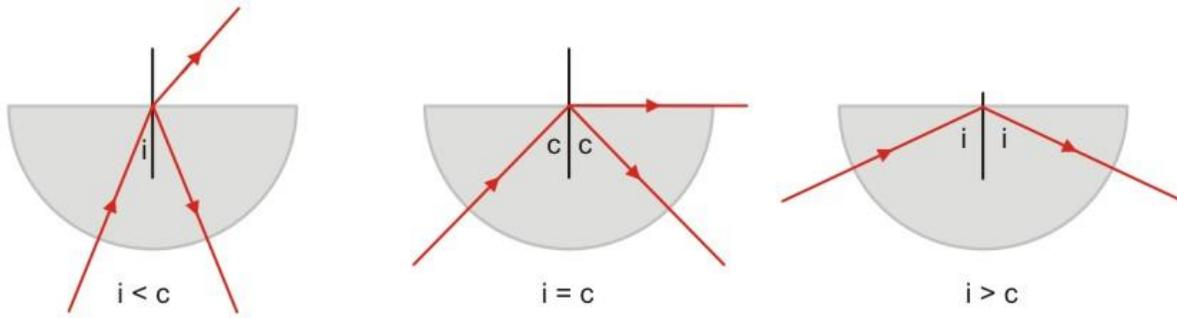
Light ray is travelling from optically denser medium to optically less dense medium.
