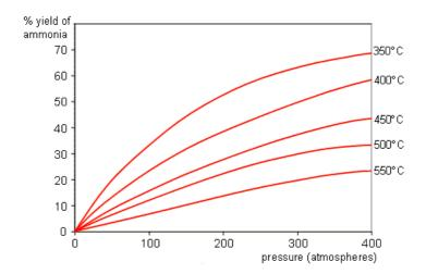
The Haber process is carried out at a **temperature of 450°C**, **pressure of 200 atm** and in the presence an iron catalyst.
