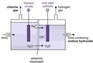
Brine is made with **concentrated sodium chloride solution**. The diaphragm allows for particles like  $Na^{\dagger}$  and  $H_2O$  molecules to pass through but does not allow negatively charged ions like  $OH^{-}$  and  $Cl^{-}$  to pass through.
