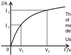
The slope of the tangent line or the gradient of *I-V* graph does not carry any physical meaning and thus cannot be used to determine the resistance of the conductor
