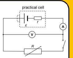
Note that the voltmeter reads the terminal voltage  $V_T$  of the batter. For the first reading:
